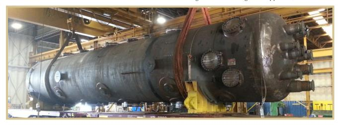
"Each of these separators is about 16.5 feet high and 15.5 feet across," Fielder explains. "They weigh about 300 tons apiece and we were tasked with engineering a loaded configuration and securement design that would enable the client to safely rail them in pairs from its plant to the waterway – a distance of about 40 miles.
