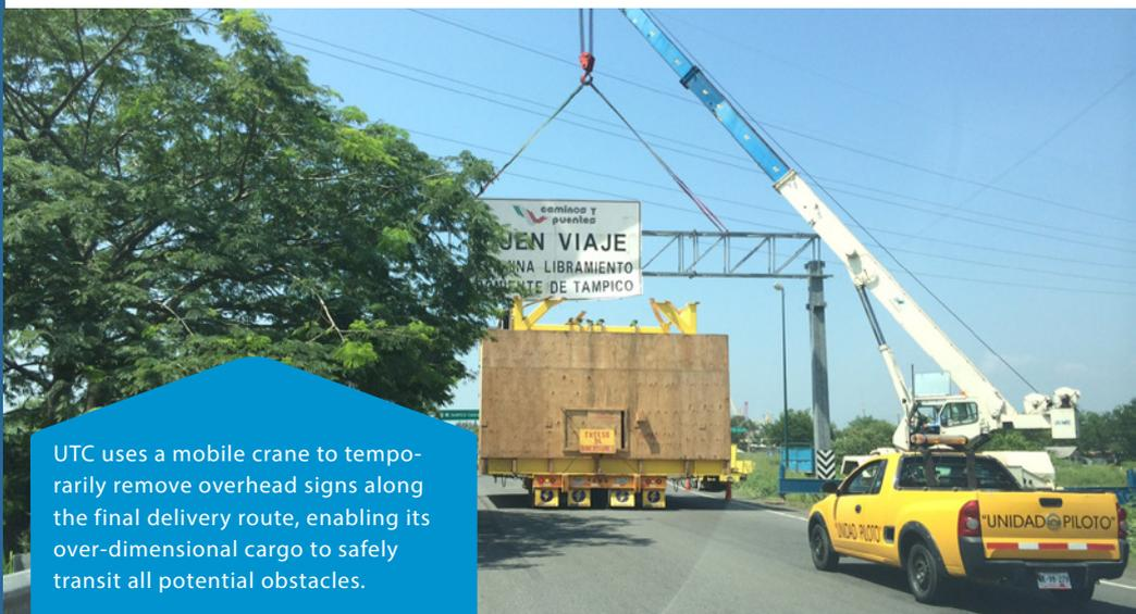
UTC uses a mobile crane to temporarily remove overhead signs along the final delivery route, enabling its over-dimensional cargo to safely transit all potential obstacles.
